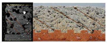
On the left: Micro-CT section; on the right: cross section of applied mortar on brick substrates
