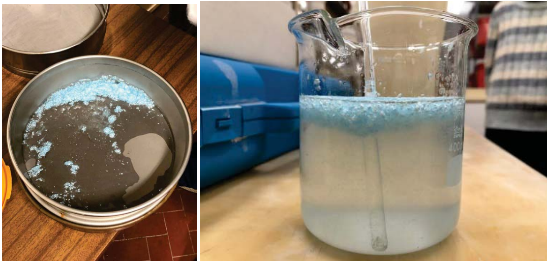
Studying the particle size (on the left) and water absorption (on the right) of mask waste
